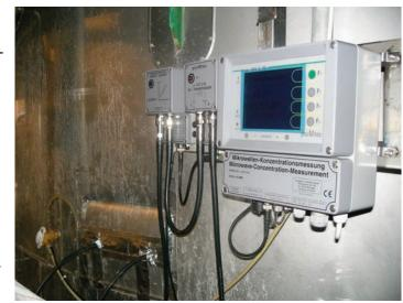
logy no bypass is there to plug and disturb the measurement. Directly immersed in the process you measure total solids content in real time and with highest possible precision.
