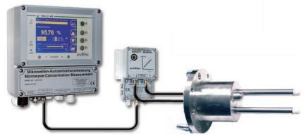
Any possible influences of temperature variations on the measurement is eliminated by a dedicated process temperature measurement in the immediate vicinity of the sensor probes.
